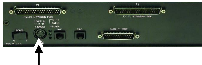
DIN5 POWER IN Connector (+10 to +30 VDC)
